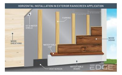
HORIZONTAL INSTALLATION DIRECT TO EXTERIOR WALL APPLICATION
