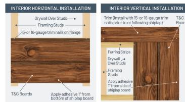
• The boards should be fastened in a similar fashion to interior wall studs. Adhesive may be used to reduce the need for fasteners.
