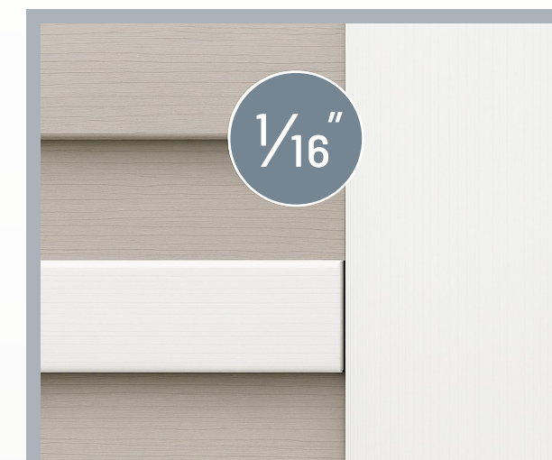
Follow gapping requirements for perpendicular trim transitions 1/16"-1/8".
